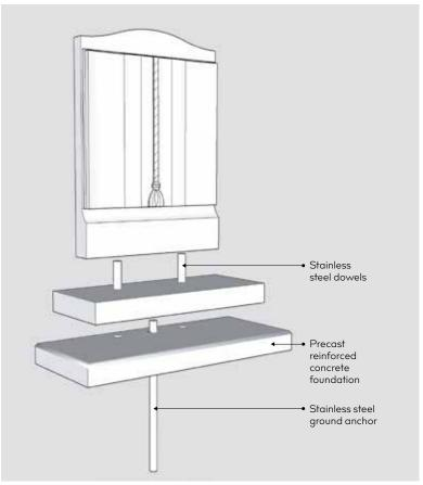
Kerb Fixing Method All sections of the memorial are securely dowelled
